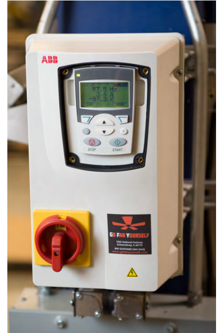
Keypad relocated to 4x4 electrical box
